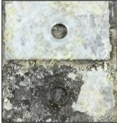
5xxx series Aluminium joined to Carbon Fiber
