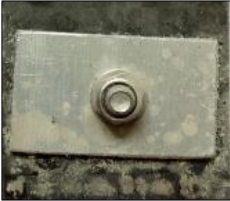
5xxx series Aluminium joined to Carbon Fiber
