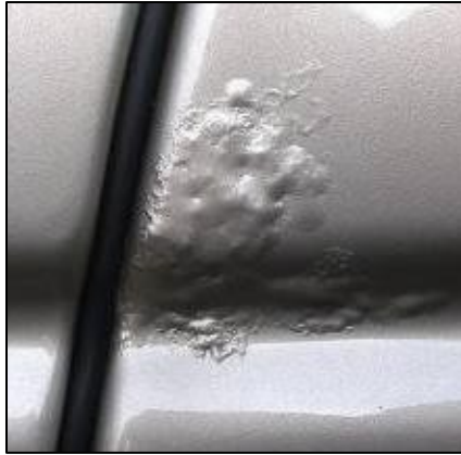
Filiform corrosion on 6xxx series painted sheet aluminium.
