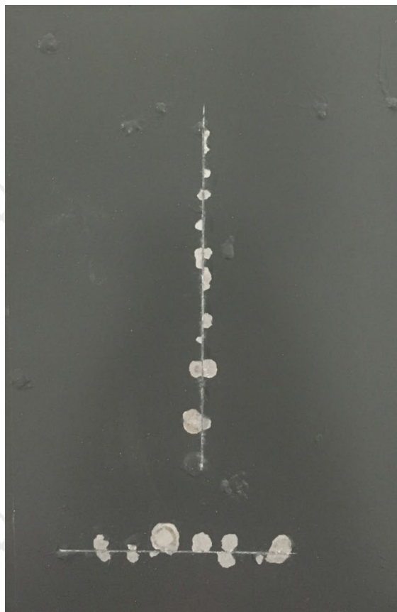
Corrosion morphology – Type C 腐蚀形貌 – 类型C
