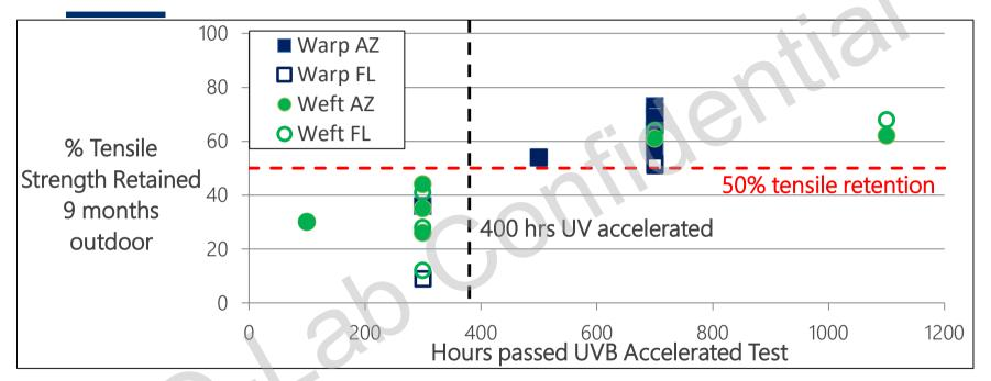
Very good pass/fail correlation between accelerated and outdoor weathering Every specimen that survived >400 hours accelerated survived 9 mo outdoors
