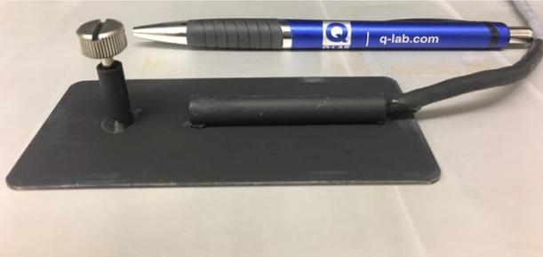
A photograph of an uninsulated black panel temperature sensor. It consists of a small black rectangular panel with a silver-colored metal mounting bracket and a black cable. A blue pen with the Q-Lab logo is placed next to it for scale.                 | 黒色塗装<br>ステンレススチール                 | Uninsulated<br>Black Panel | Black Panel       |
