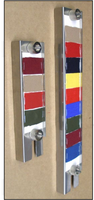
Textile Specimens on cardstock in Xe-2 holder
