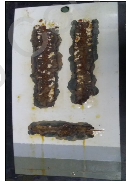
Steel panels: CATCH - 1728 h (from left to right: good, middle, bad)
