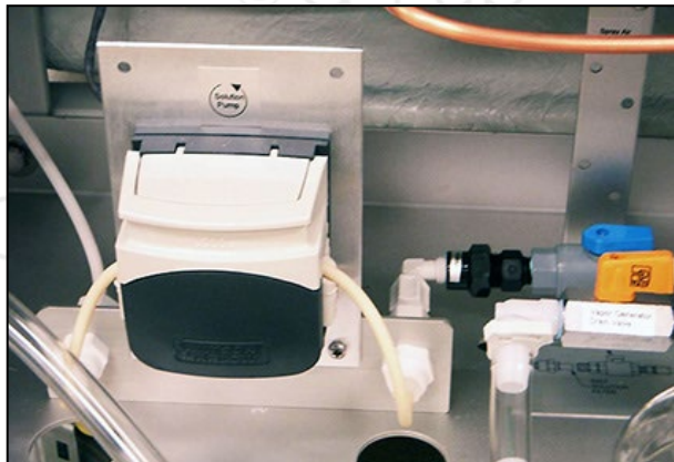
Solution Pump Speed 30-40%
