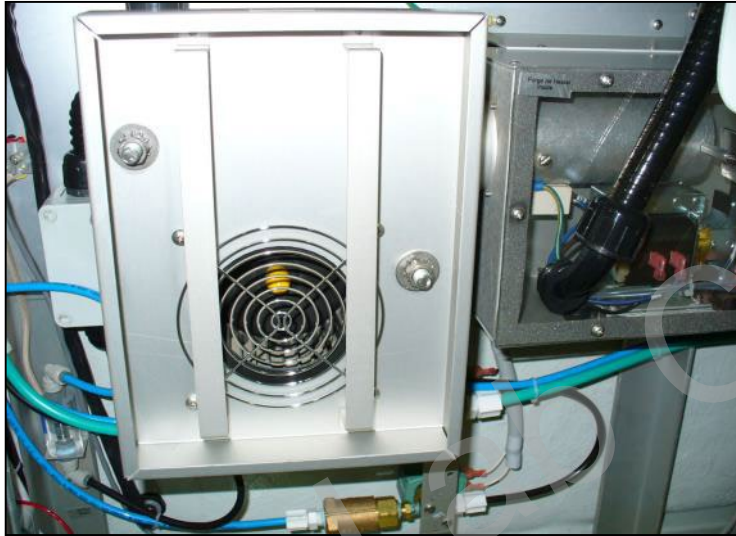
Purge Air Blower
