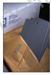
**Q-PANEL** are the World's Most Widely Used Test Substrate for Paints
