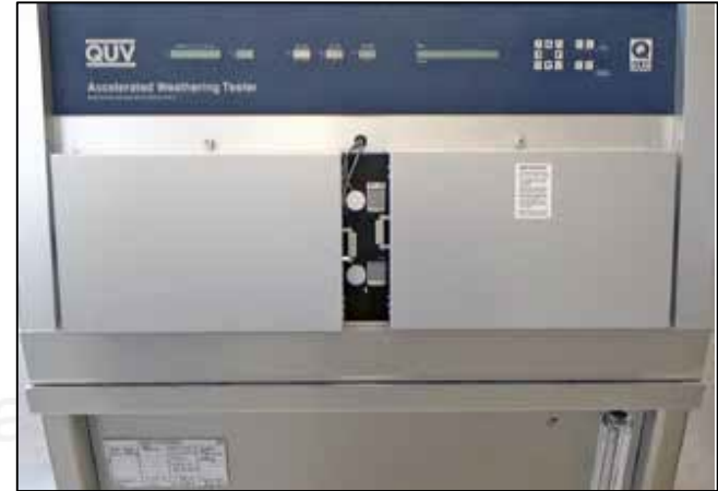
QUV with door removed and 3D Boxes
