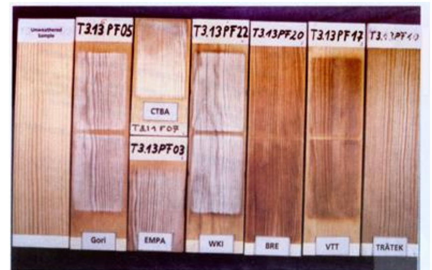
Photo 2: System F at the end of the seven exposure cycles.
